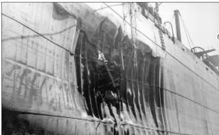
TORPEDO EXPLOSION DAMAGE TO PORT LOWER SIDE OF HULL OF SS FORT CAMSON . (LAC PA190186)
